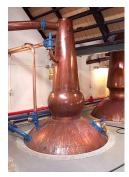
angled lyne arms which descend into worm tubs. The spirit stills are small with flat tops and a long, gently angled lyne arm sticking out of the side of the still. They too end up in worms. It is the latter pair – the only such type in Scotland – which help to generate the make's complexity.
