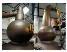
to separate specific alcohols. The spirit still has both a purifier pipe and a very convoluted, coiling lyne arm. Again, reflux is maximized here, with that purifier conceivably adding oiliness to the character. Condensing takes place in worm tubs which add weight.
