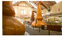
Glenfarclas has resisted changing their production methods as indicated by their retention of direct fire. Steam heating was tried in 1981, but the conclusion was that the guts went out of the new make spirit, and direct fire went back in; after all, a rich distillate is needed to cope with the tannic structure and rich fruits of ex-Sherry casks.
